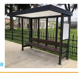
BRTA bus shelters were retrofitted with materials from SABIC to test durability, scratch resistance, and ease in graffiti cleanup. Two test shelters in the heavily used, main thoroughfare of Downtown Pittsfield were retrofitted to provide feedback on what worked well and what needed some improvements in order to survive this harsh environment.
